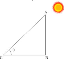
From the figure, it is clear that △△ABC is a right-angled triangle in which AB is the vertical rod and BC is its shadow.
